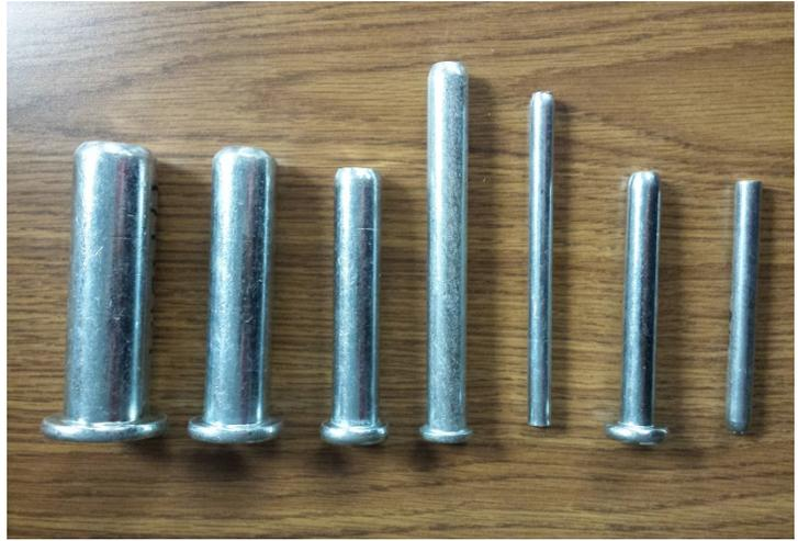
A sample of pins used in pin-connected trusses.
