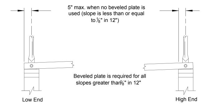
Beveled plate is required for all slopes when trusses are cantilevered
