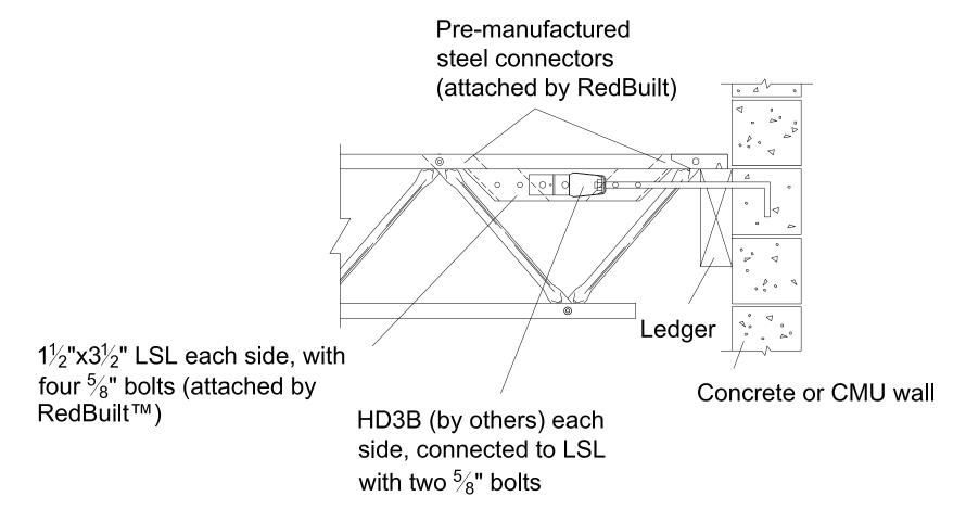
Truss assembly tension capacity is 4,450 lbs at 133% or 160%. Minimum truss depth is 15" and maaximum slope is  $\frac{1}{2}$ " in 12. (Wall and anchorage design by others.)
