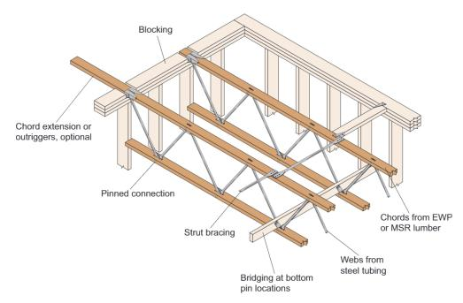
Example diagram of pin-connected trusses.
