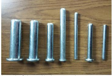
A sample of pins used in pin-connected trusses. From L to R: 1.25", 1.0", 0.75", 5/8", 3/8", 1/2" and 3/8".
