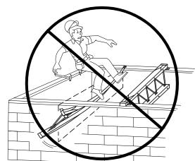
DO NOT walk on the trusses until all truss bearings and bracing have been permanently attached.
