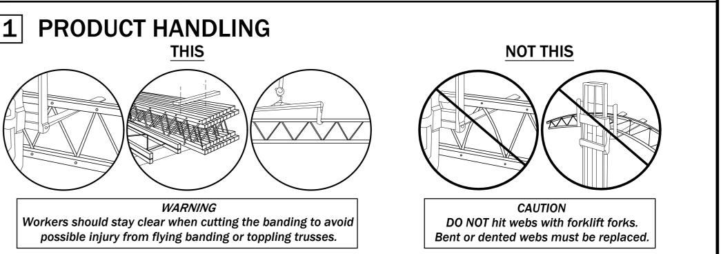
Trusses will be delivered to the jobsite in bundles of twenty or fewer, banded together for handling and shipment. To avoid damage they should be left in these bundles until they are ready to be installed in the structure. Miscellaneous hardware such as bearing angles, lag screws, bolts and nails as required for each specific job will be shipped in bags or boxes with the trusses.
