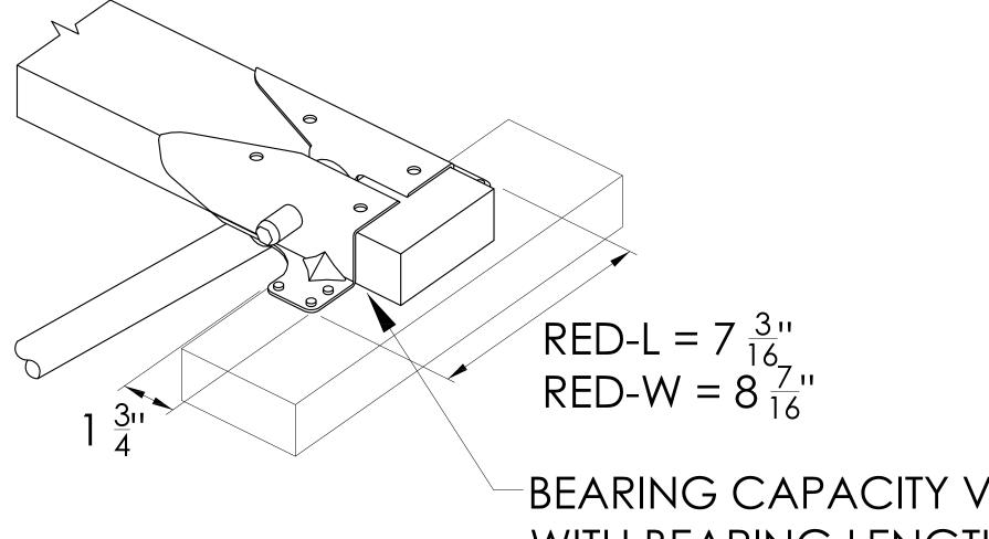
BEARING CAPACITY VARIES WITH BEARING LENGTH
