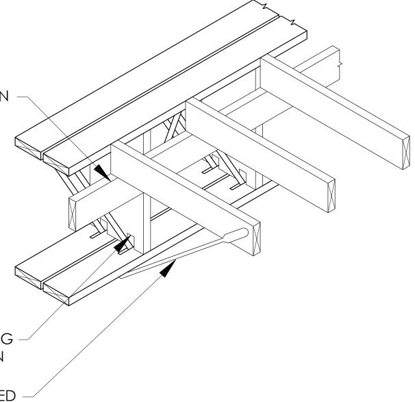
LOAD TRANSFER BLOCK SPACING VARIES BASED ON TRUSS DESIGN
