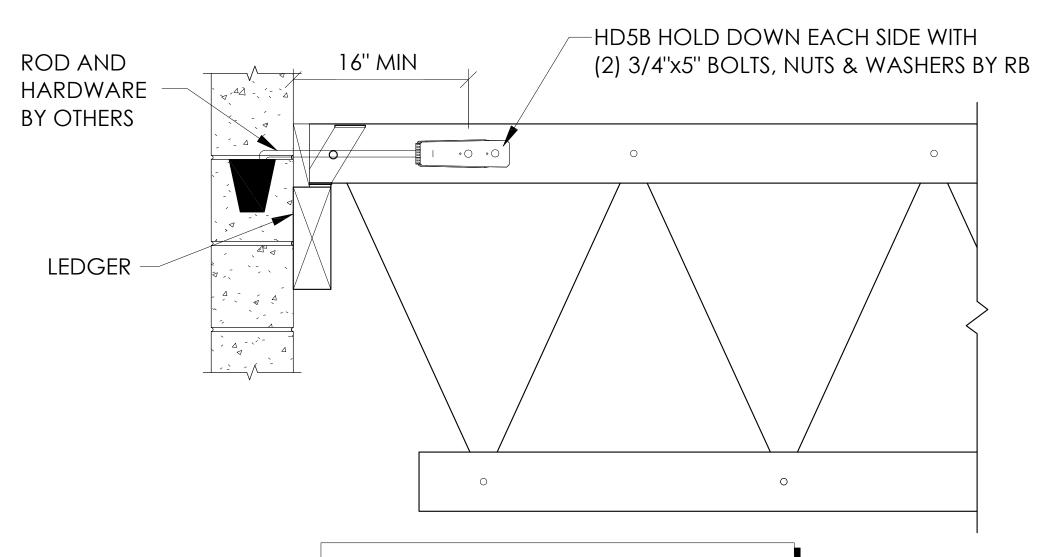
THE DESIGN PROFESSIONAL OF RECORD IS RESPONSIBLE FOR THE ROD TO HARDWARE AND CONCRETE/CMU CONNECTIONS
